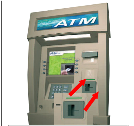
Criminal installs skimming device and camera on ATM
