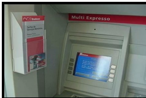
Small camera attached to brochure holder to capture PIN
