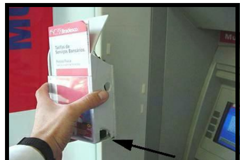
Small camera attached to brochure holder to capture PIN
