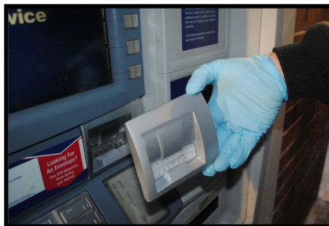
Skimmer attached over actual card reader
